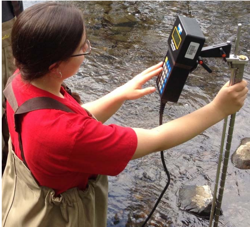
Maya Domeshek '18 takes a discharge measurement downstream from Paradise Pond.
