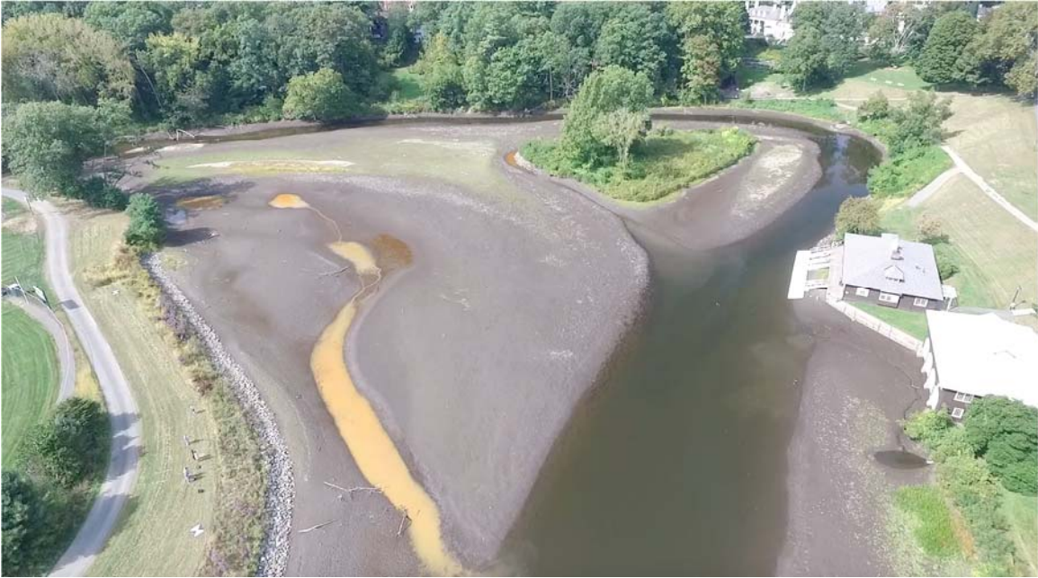
Drone image of sediment-filled Paradise Pond bottom exposed during a partial drawdown in September 2015. (See Section 4.1 for more on the Paradise Pond sluicing project)
