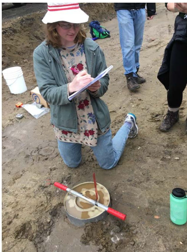
Tessa McGann '16 measures infiltration capacity during a geoscience class at the Mandelle site.
